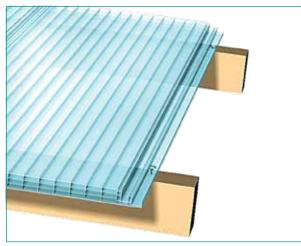
Fix the panel with a screw on each rafter.
