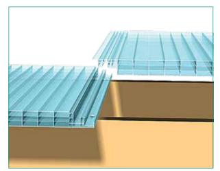
Join the next panel, taking care to match the male / female profiles before applying pressure. Ensure that panel is fixed.
